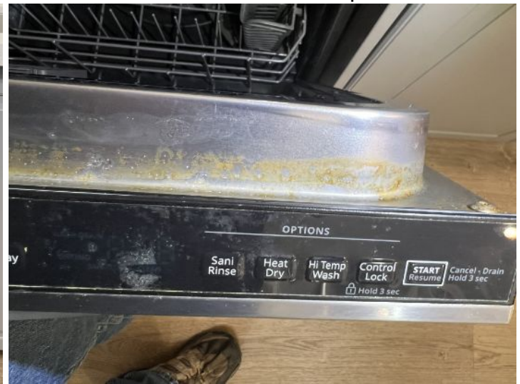
Corrosion at the top
