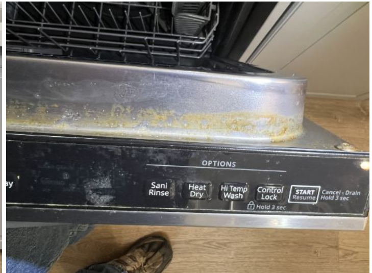
Corrosion at the top
